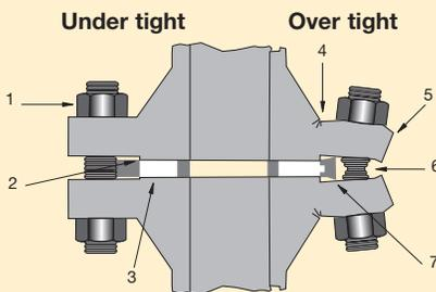
1. Bolt loosens due to cycle loads of vibration.
