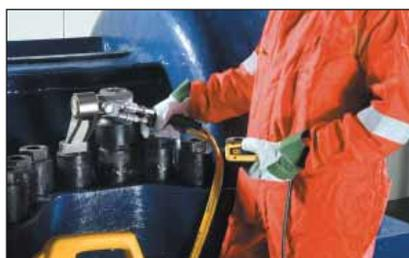
◀ Any brand of hydraulic torque wrench can be powered by the portable ZU4-Series torque wrench pump.
