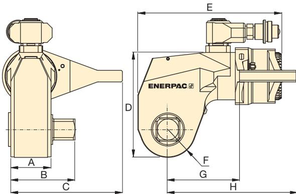
The rigid steel design of S-Series torque wrenches guarantee durability, reliability and safety. These wrenches can be powered by the portable ZU4T-Series pumps.
