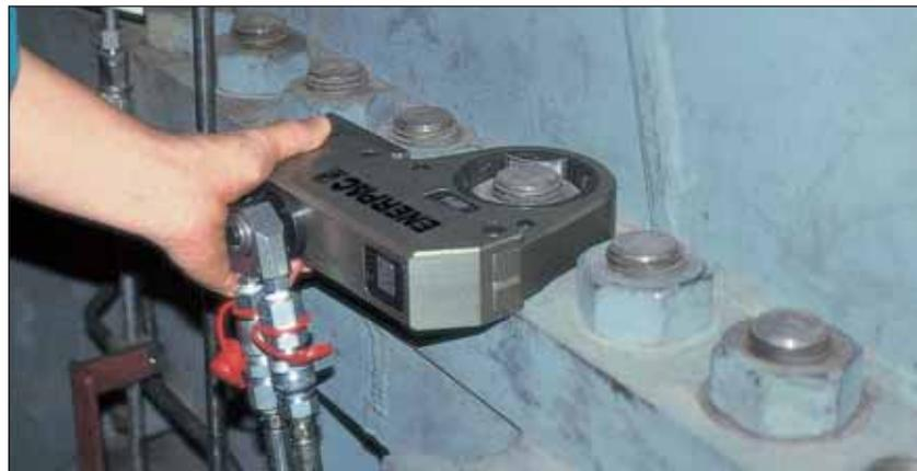
▼ An Enerpac HXD hydraulic wrench brings safety and efficiency to this flange maintenance job at a refinery.
