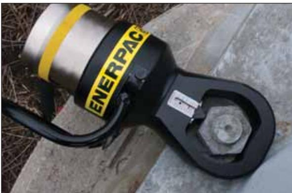
◀ Heavily corroded and weathered nuts are quickly split and removed using an NS-Series Nut Splitter.
