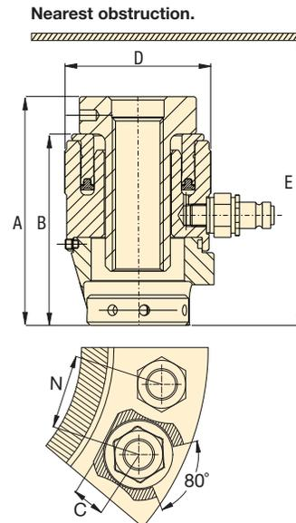
▼ GT2 Bolt Tensioner on a flange joint.
