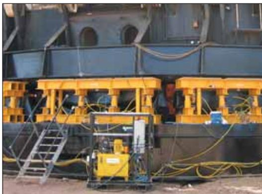
◀ Positioning a 3500 ton dragline was successfully done with an Enerpac synchronous system. This operation provided for exact alignment of the bearing on the rail, prior to torque tightening of the slew ring bolts.
